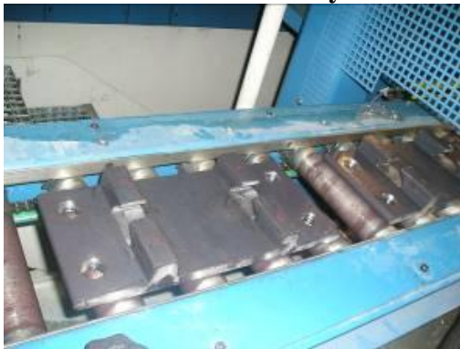
A detail of the roller conveyor with workpieces
