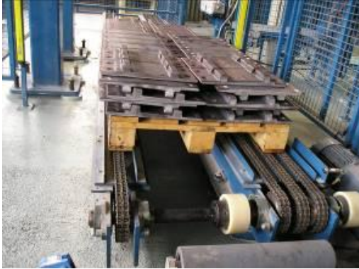
A detail of the pallet conveyor with workpieces
