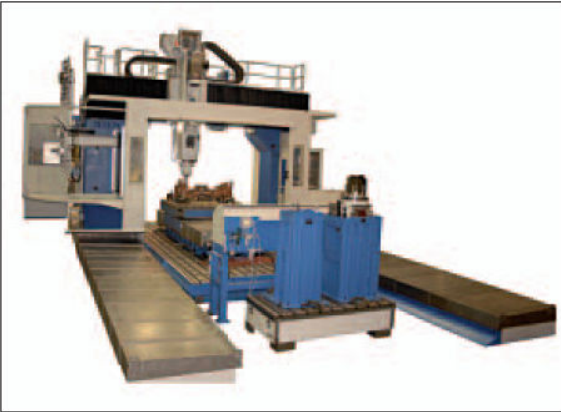
FRUQ portal milling machines will soon get their 60 kW headstocks too
